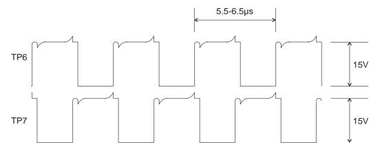
Figure 6.1 TP6 & TP7 Voltage Waveforms
